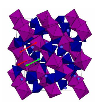
Lattice displacements giving rise to magnetoelectric effect in Tb<sub>3</sub>Fe<sub>5</sub>O<sub>12</sub>
